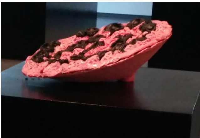
Figure 2. The Silicone Valley . The black hard plastic elements protruding from the breast tissue concentrate the vibration feedback and host the conductive copper wire of capacitive sensors.
